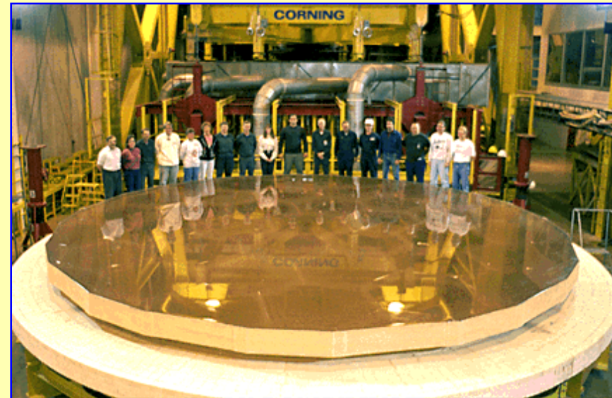
First 8-m mirror blank for the Gemini project. The mirror blanks are manufactured by fusing hexagonal pieces of ULE zero-expansion glass in a high-temperature furnace.
